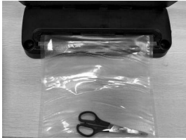
One side of the bag on the sealing line
